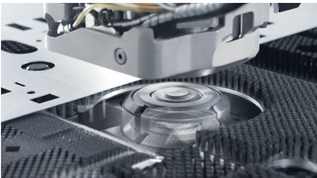
The active die provides for active reshaping from below and enables scratch-free processing.
