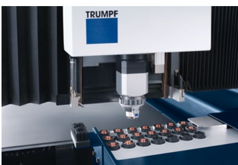
Save even more time with options such as the automatic nozzle changer.
