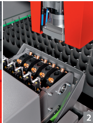
1 Cutting head 2 Nozzle changer 3 Operator panel with ByVision Cutting
